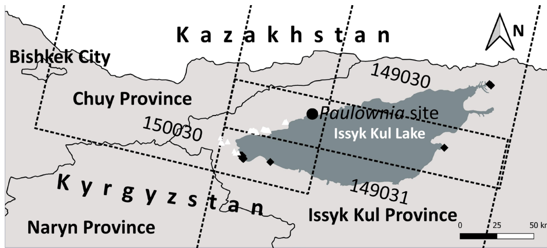
Figure 1. Map of Issyk Kul Lake, including neighboring areas, and locations of the Paulownia site (black circle), cold pixels (black diamonds), and hot pixels (white triangles). The dotted lines and inclined numbers refer to the Landsat tiles with their respective path and row numbers.
